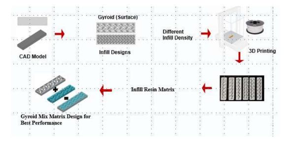
Model structures were printed using Thermoplastic Polyurethane Gyroid structure with infill epoxy resin as shown below.
