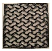
3-point bend test were performed on various 3-D printed gyroid composite panels are shown below
