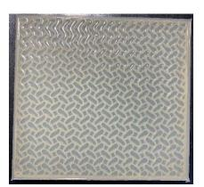
Model structures were printed using Thermoplastic Nylon (polyamide) Gyroid structure with infill epoxy resin as shown below.
