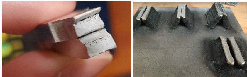
Figure 1: Internal porosity present in ZX (vertical) dogbone sample and overhang benchmark structures. Weld beads collapse on themselves on overhang angles greater than 45 degrees.
