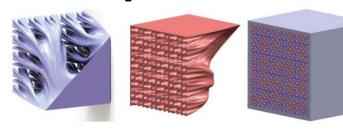
The design shown above [1] is a thermally optimal design for a heat exchanger as studied by Uwe Scheithauer, Richard Kordaß, and peers. We propose this structure to be in the inner lattice of the phone case for optimal heat distribution.
