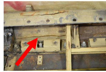
Stress-corrosion cracking of high-hard steels
