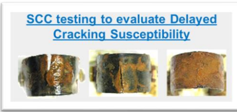
Stress-corrosion cracking of high-hard steels
